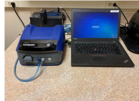
Fig. 8. PortaCount® quantitative fit test device.
